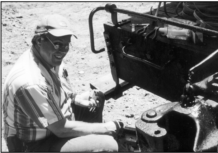
Mike Gailus installs an electric box and plug on the tie below the rear steps of the tender. – Photo © Bob Tully.
